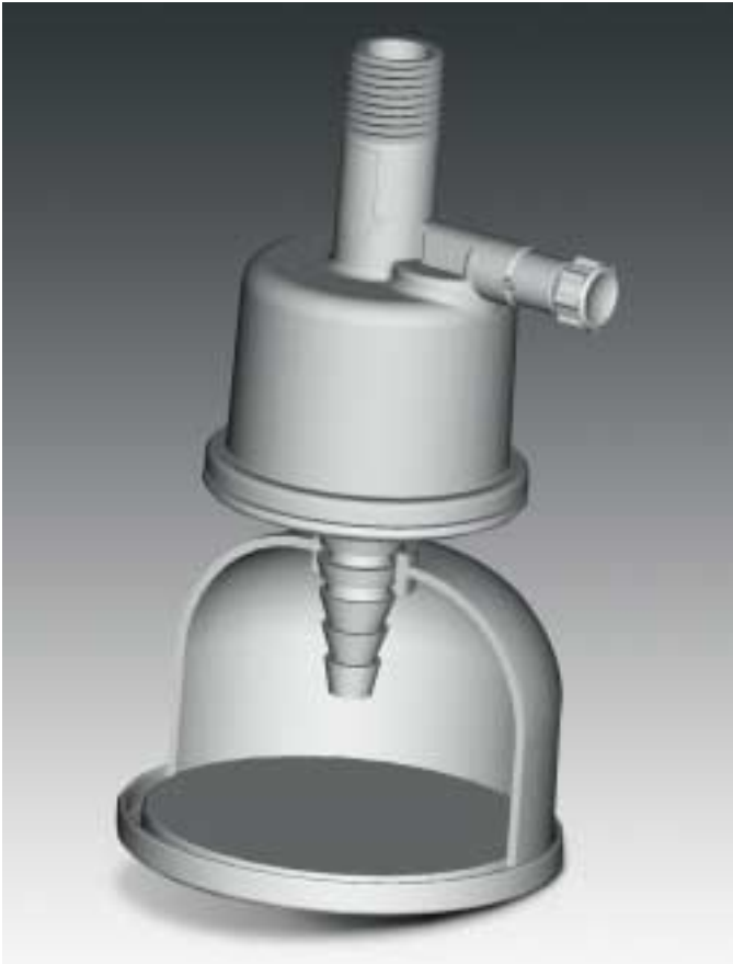
CAD rendering of Sartopore 2 150, with cut-away of filling bell.
