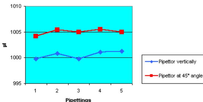
Fig. 2. Comparison of the pipetting results when the pipettor is held vertically and approximately at 45° angle. As seen, pipetting at an angle increases the volume.
